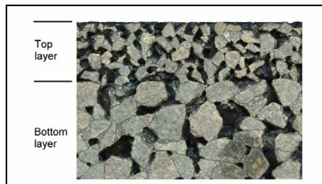
Figure 7: Structure of double-layered Porous Asphalt
